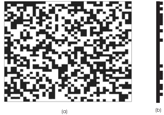
Fig. 1. Front and side view of a RPP with square zones. Black and white zones are in reality equally transparent, but white zones do not introduce additional phase, black zones introduce an additional phase of \lambda/2 . Hence only the phase of the initial beam (and not the intensity) is damaged which explain the name of “phase plate”.
